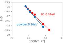
Activation energy of diffusion motion. (An Arrhenius plot of diffusion coefficient)
