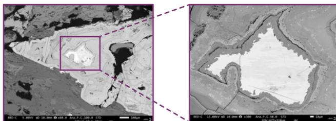
In this study, BSE imaging allows to see the **difference of chemical composition** on the observed area. Thus, this study area showing **important contrasts**, sign of **important chemical variation**, is selecting for additional on complementary analysis.
