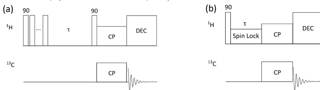
Fig.1 Pulse sequence diagrams of saturation recovery ( $T_1^{\text{H}}$ ) based ROSY(a) and spinlock ( $T_{1\rho}^{\text{H}}$ ) based ROSY(b).
