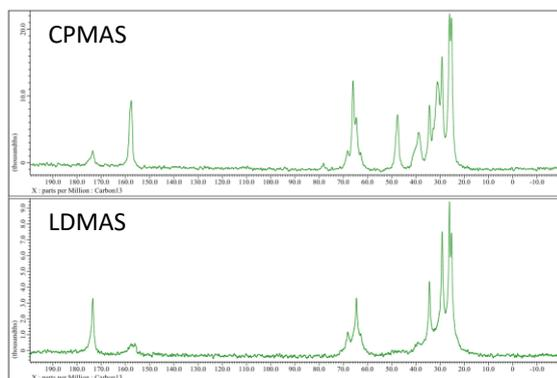
Fig.2  $^{13}\text{C}$  CPMAS and LDMAS spectra of poly urethane.
