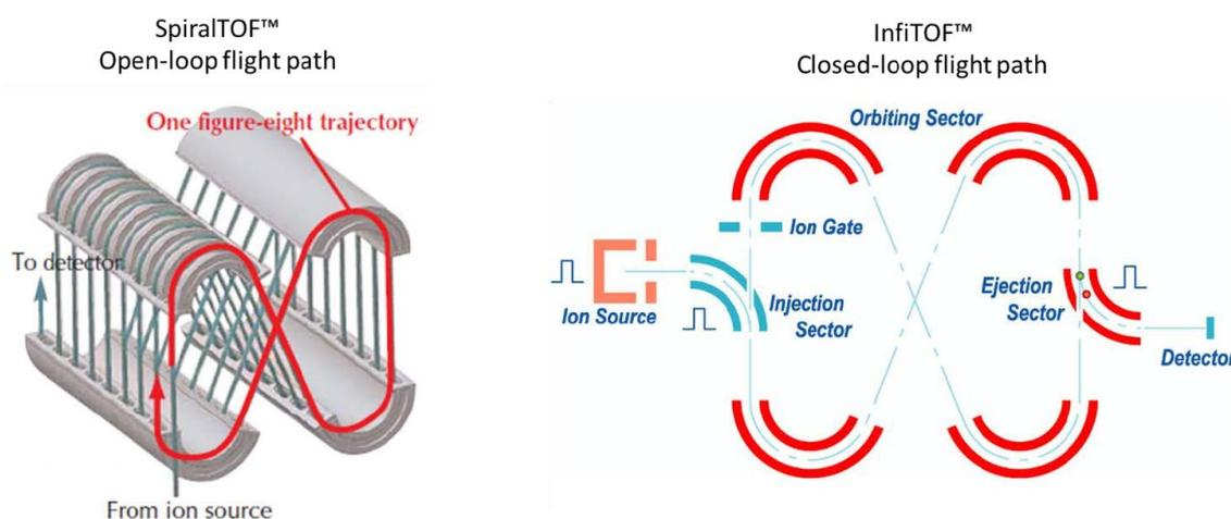
Figure 2. Two multi-turn mass spectrometer configurations.
