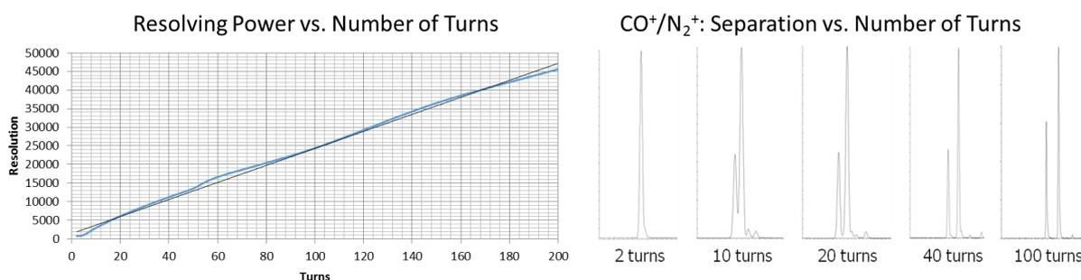
Figure 3. Mass resolving power increases with multiple turns around the InfiTOF ion optics.
