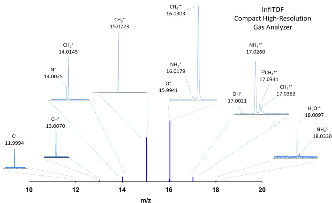
Figure 5. High-resolution InfiTOF mass spectrum of 5% ammonia in methane.
