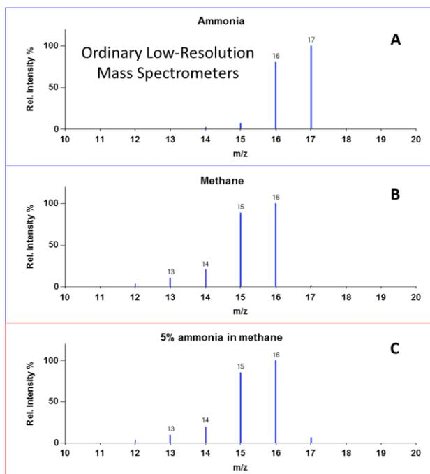
Figure 4. Low-resolution electron ionization (EI) mass spectra of ammonia (A) and methane (B) and a 5% mixture of ammonia in methane (C).
