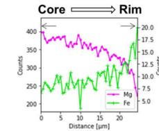
Fig.4: The X-ray intensity of Mg and Fe in the grain at the center.
