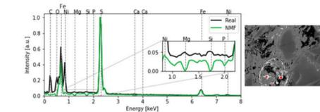
Fig.7: The NMF component and real EDS spectrum corresponding to Fe, Ni-sulfides.
