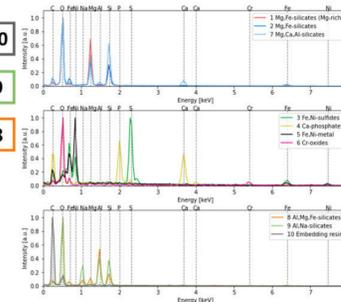
Fig.2: X-ray spectrum of each area. Compound name in the legend are based on the quantitative analysis results. Acc. Vol. 10 kV.
