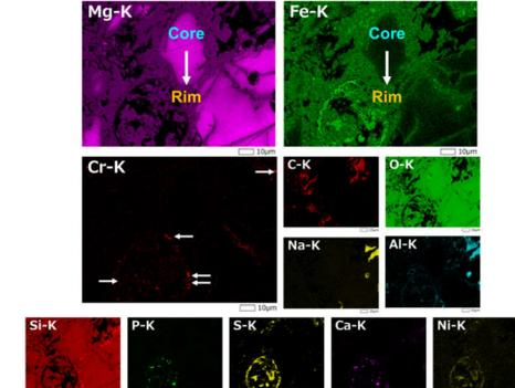
Fig.3: The elemental maps of the sample. Cr is sparsely located, as indicated by arrows. Acc. Vol. 10 kV. EDS map size: 256x192 pixels.
