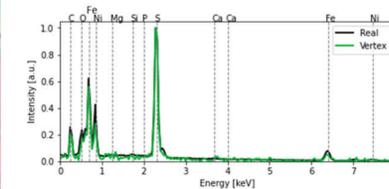
Fig.10: The vertex spectrum and real EDS spectrum corresponding to Fe, Ni-sulfides. Vertex spectrum (green): obtained by VCA. Real (black): same as real EDS spectrum in Fig.7.
