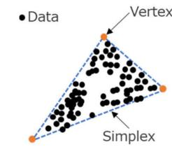
Fig.8: Conceptual Diagram of VCA. VCA is an algorithm that finds the vertices from simplex-shaped dataset. The vertices of SI can be used for unmixing SI by its own signature spectra.
